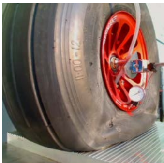
← ↑ 440,00lbs Hydraulic press for ultimate load tests
